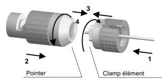
Solder the cable inner conductor into
